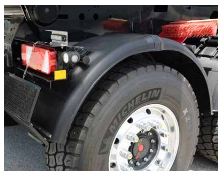
Sturdy fixtures for the mudguards are indispensable for use on the construction site.
